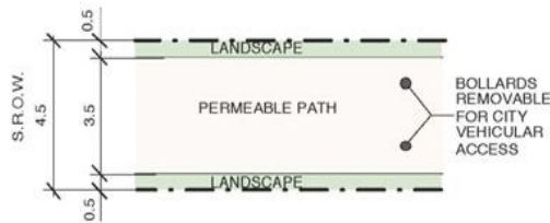
4 FORESHORE PATH ACCESS MULTIPURPOSE (BIKE, PEDESTRIAN), AND CITY SERVICE ACCESS (3 LOCATIONS - EAST AND WEST)
