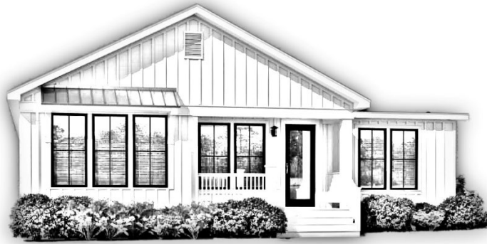
Figure 6 - Example of Modular Home – a modular home can take many forms, however, is constructed on site from factory assembled modules
